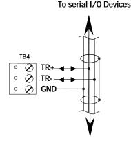
*Important:* Install the termination jumper ONLY on the panel at each end of the RS-485 bus. Failure to do so will compromise the proper operation of the communication channel.
