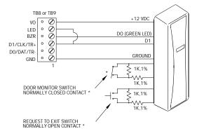
\* Jumper: Connect D1 and LED on supervised F/2F readers.
